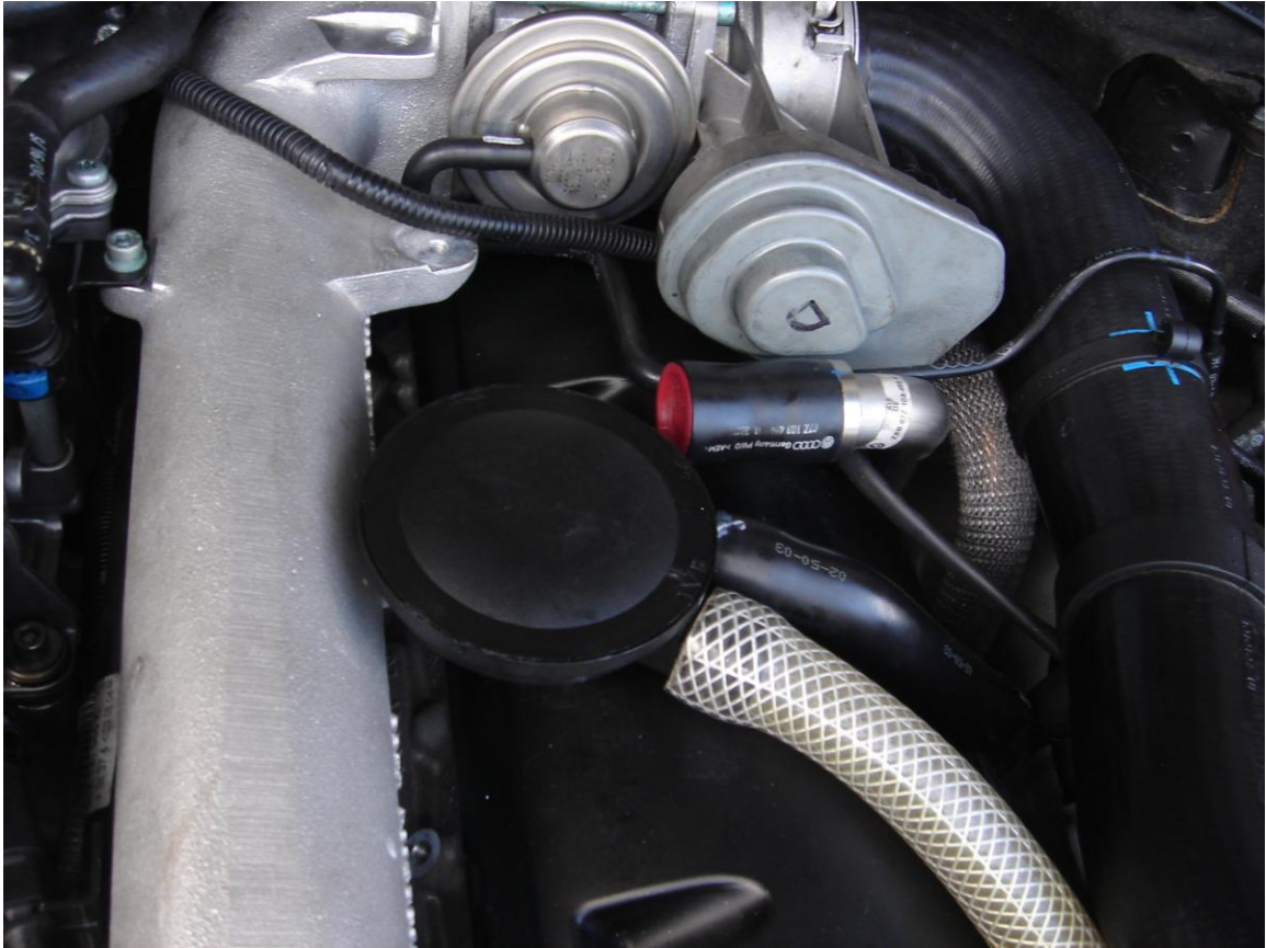
P-side CCV valve on the D-side, capped intake tube.
