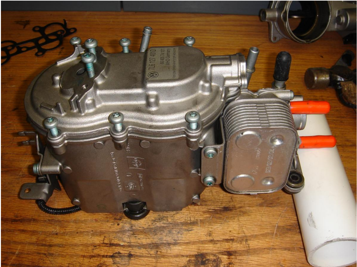
Fuel Filter/heat exchanger out of the car.
