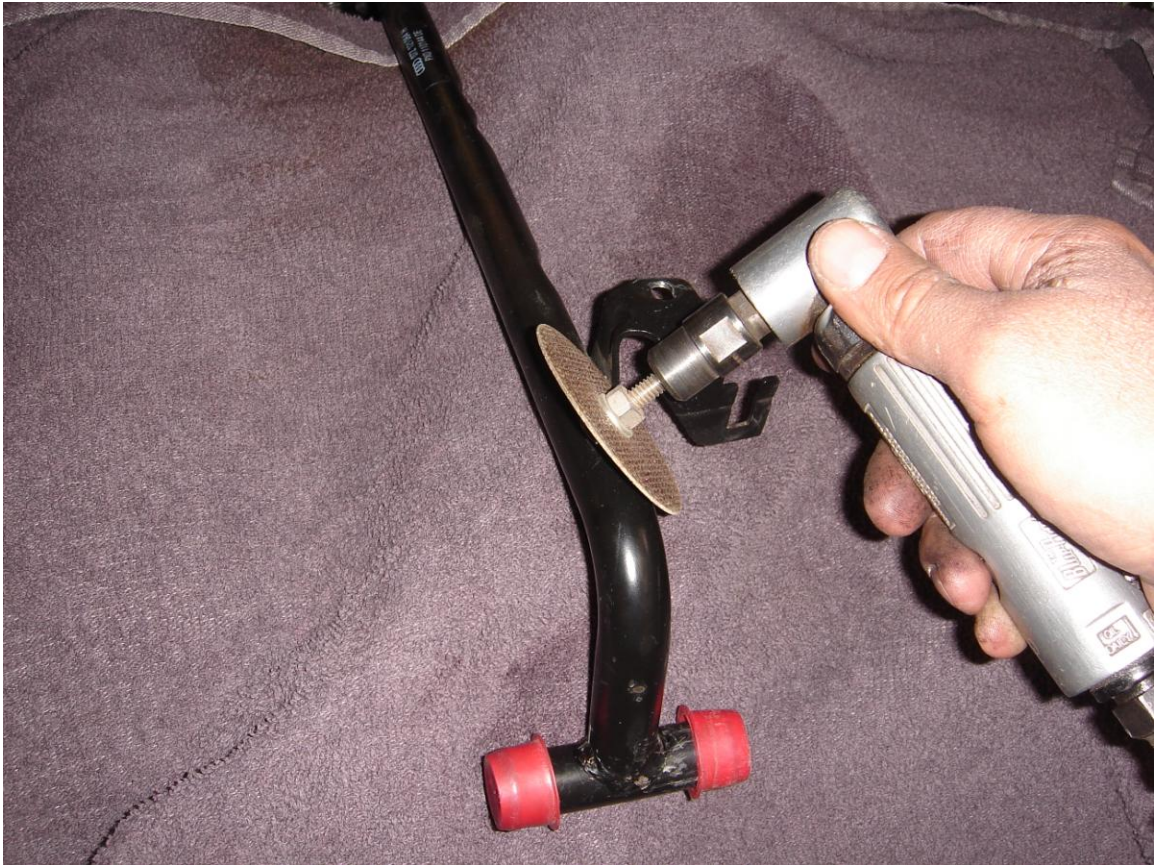
Cutting the troublesome bracket off of the T-pipe
